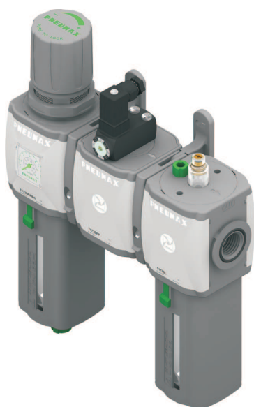
Example : GT173BRG : size 3 combined group comprising Filter-Regulator, Pressure switch and Lubricator Technopolymer threads, G1/2" connections 0 to 8 bar adjusting range and 20 µm filter pore size
