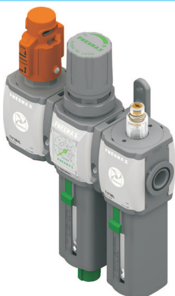
Example : GT171BVHG : Size 1 Combined group comprising Shut-off valve, Filter-regulator and Lubricator Technopolymer threads, G1/4" connections 0 to 8 bar adjusting range and 20 µm filter pore size
