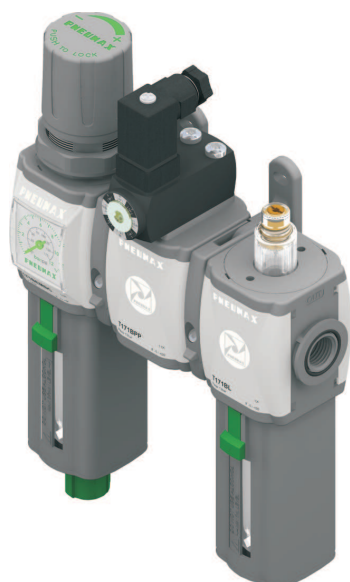
Example : GT171BRG : size 1 combined group comprising Filter-Regulator, Pressure switch and Lubricator Technopolymer threads, G1/4" connections 0 to 8 bar adjusting range and 20 µm filter pore size
