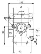
Weight 3178 g Normally closed Minimum actuation pressure 2 bar
