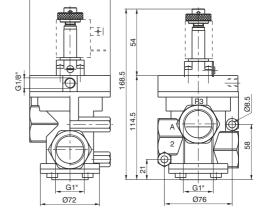
Weight 1120 g Minimum actuation pressure 2 bar
