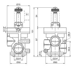
Weight 1160 g Minimum actuation pressure 2 bar
