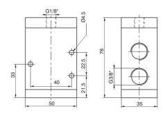
Weight 360 g Minimum actuation pressure 2 bar
