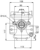
Weight 3168 g Normally closed / Normally open Minimum actuation pressure 2 bar
