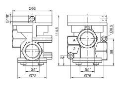
Weight 1060 g Minimum actuation pressure 2 bar
