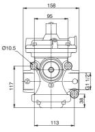
Weight 3238 g Minimum actuation pressure 2 bar
