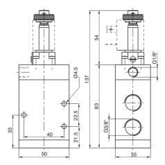
Weight 420 g Minimum actuation pressure 2 bar
