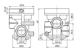
Weight 990 g Minimum actuation pressure 2 bar
