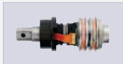
The strain gauges are positioned on the main shaft, picking up the twisting torque on the main shaft at each impulse as close as possible to the socket. The electric signals are transmitted by induction through the internal and external coils. Due to this principle the YOKOTA transducer is very reliable, accurate and without wear. The angle sensor is also mounted on the main shaft.
