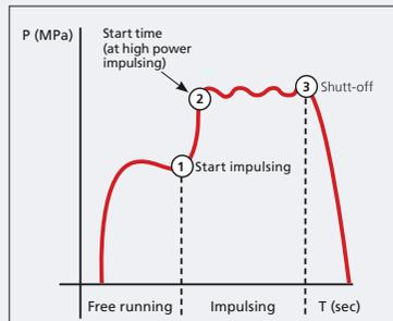
The whole system is more accurate than shut-off or standard impulse wrenches.
