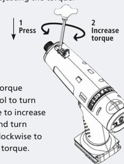
2. Use the torque adjust tool to turn clockwise to increase torque and turn counterclockwise to decrease torque.
