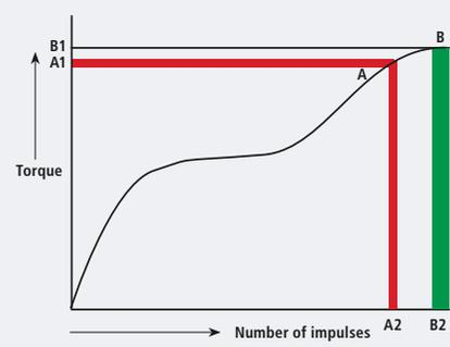
**A** = shut-off area of mechanical shut-off impulse wrenches
