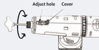
1. Lift the torque adjustment over. Take the torque adjust tool and insert it to the quick change holder and turn until the adjust hole shows up.
