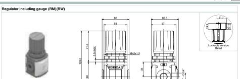
Example: T172BRMC: size 2, Regulator including gauge with Technopolymer threads, G3/8" connections, 0 to 8 bar adjusting range
