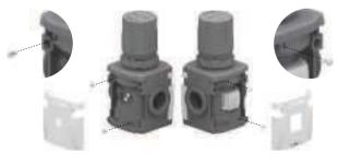
Bowls, plugs and supports are assembled with a bayonet type mechanism. In order to remove them rotate anti-clockwise until you reach a mechanical stop, then remove from the component body (For bowls, firstly press down the green safety button). Please note: Bowls and transparent parts can be cleaned with water and neutral soap. DO NOT USE SOLVENTS OR ALCOHOL
