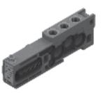
In particular this module is fitted with a M8 3 pins connector: +24V. not connected. GND.
