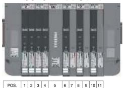
PIN 1 = PILOT 14 EV POS.1 PIN 2 = PILOT 12 EV POS.1 PIN 3 = PILOT 14 EV POS.2 PIN 4 = PILOT 12 EV POS.2 PIN 5 = PILOT 14 EV POS.3 PIN 6 = PILOT 14 EV POS.4 PIN 7 = PILOT 14 EV POS.6 PIN 8 = NOT CONNECTED PIN 9 = NOT CONNECTED PIN 10 = NOT CONNECTED PIN 11 = PILOT 14 EV POS.8 PIN 12 = PILOT 12 EV POS.8 PIN 13 = NOT CONNECTED PIN 14 = NOT CONNECTED PIN 15 = PILOT 14 EV POS.10 PIN 16 = NOT CONNECTED
