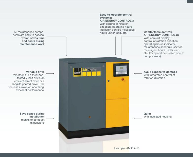
The solution for permanent air requirements, e.g. spray painting or industrial manufacturing applications. AirMaster screw compressors ensure easy servicing, silent operation and greater operating comfort from a clearly laid out control system that is simple to use.
