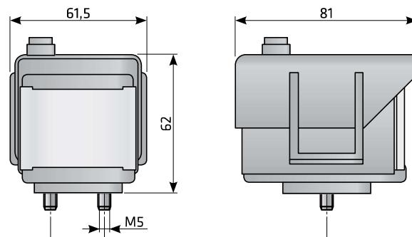
**MDH****DIFFERENTIAL HIGH PRESSURE INDICATOR**operating pressure **50 bar**operating temp. range **1,5 to 65 °C****APPLICATIONS**
