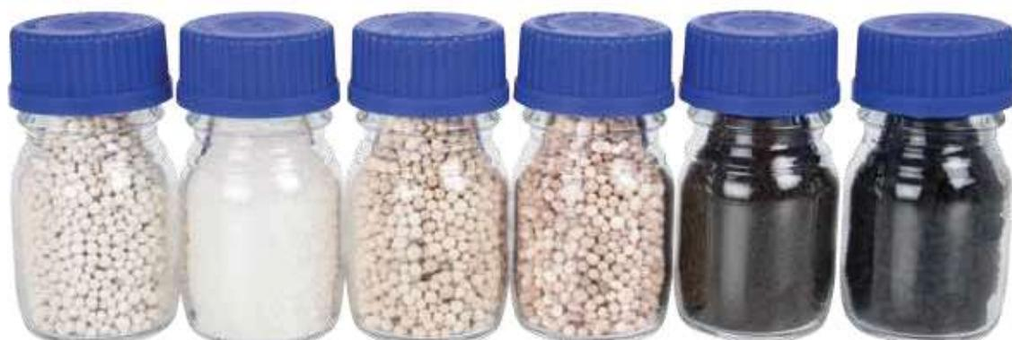
**Molecular sieve 3A** - drying of unsaturated hydrocarbons
