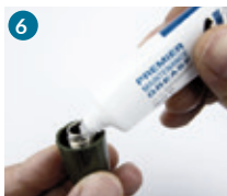
6 Grease the threads of fluid adjustment knob
