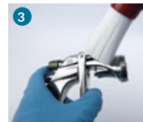
3 Clean the spray gun surface
