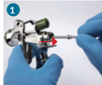
1 Remove the needle adjustment knob and needle spring
