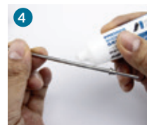
4 Grease the needle
