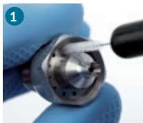
1 Clean the fluid nozzle small holes with a tiny twisted brush \varnothing 3 mm
