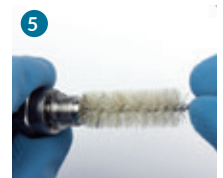
5 Clean smoothly the internal nozzle part, by using the most suitable brush size
