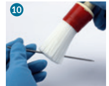
10 Clean the fluid needle with the most suitable brush
