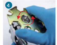
4 Unscrew and remove the fluid nozzle by the universal spanner
