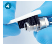
4 Clean carefully the nozzle threads with a brush
