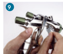
9 Adjust needle packing (15-60 degree tighten), by using the special spanner
