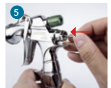
5 Insert the fluid needle in its seat
