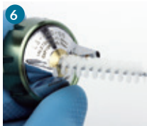
6 Clean the air cap center hole with the most suitable twisted brush size
