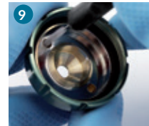
9 Clean the rear air cap holes with the most suitable cleaning needle size
