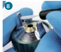
8 Clean the air cap horn holes with the most suitable cleaning needle size
