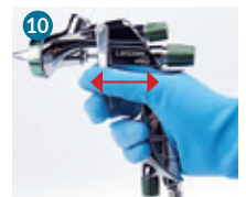
10 Check if the trigger glide is smoothly.
