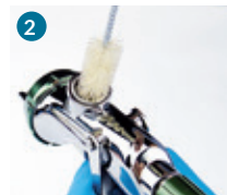
2 Clean the passages of the fluid, by using a blow gun and a twisted brush \varnothing 10 mm
