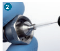
2 Clean the central nozzle orifice with a tiny twisted brush \varnothing 3 mm
