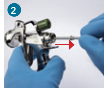
2 Take out the fluid needle
