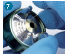
7 Clean the tiny air cap holes with the most suitable cleaning needles size
