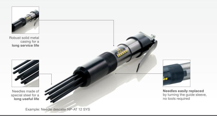
The needle descalers with metal housing have an impressively long service life and are fitted with extremely durable needles made from special steel. Ideally suited for removing coarse rust, welding cinder and paint, processing stone, fettling welded seams, roughing surfaces and removing residual plaster and concrete from reinforcing steel.
