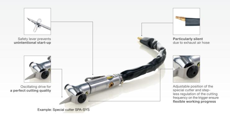
The special cutter is suitable for removing vehicle windscreens stuck in position. The oscillating cutter is ideal for removing wax, sealant and underbody protection.
