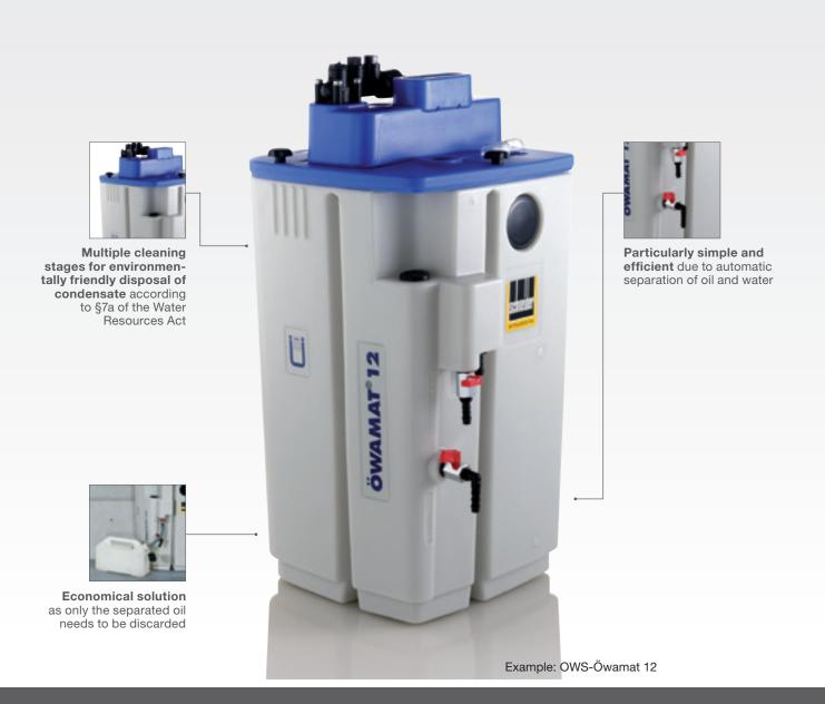
Oil-water separators use an automatic separation process and multiple-stage cleaning process to purify condensate containing oil. They represent an environmentally friendly cost-saving solution for separating condensate and allow the oil to be discharged into the sewage system as specified in §7a of the Water Resources Act.
