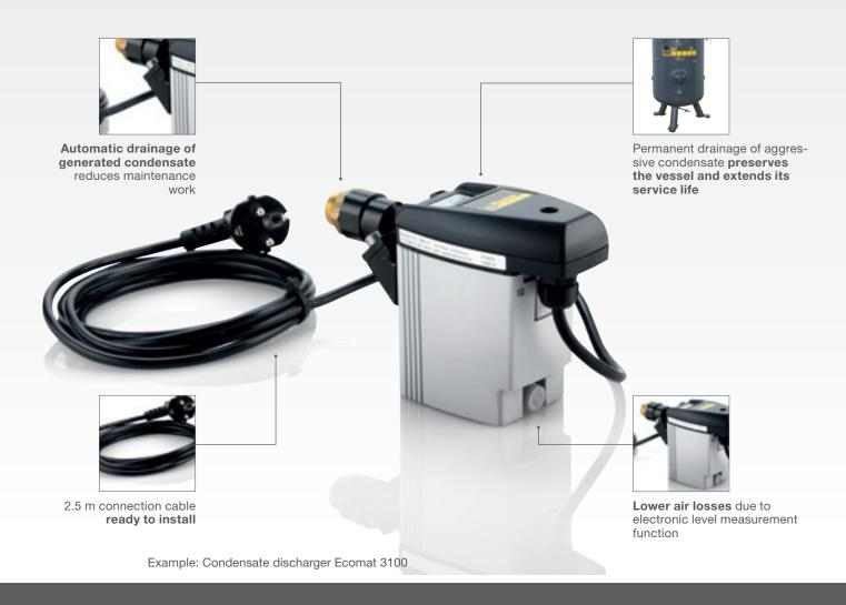
Condensate dischargers automatically discharge the condensate from vessels, filters and compressed air dryers. The dischargers are extremely low-maintenance due to the electronic level measurement function and are suitable for compressed air systems up to 15 bar.
