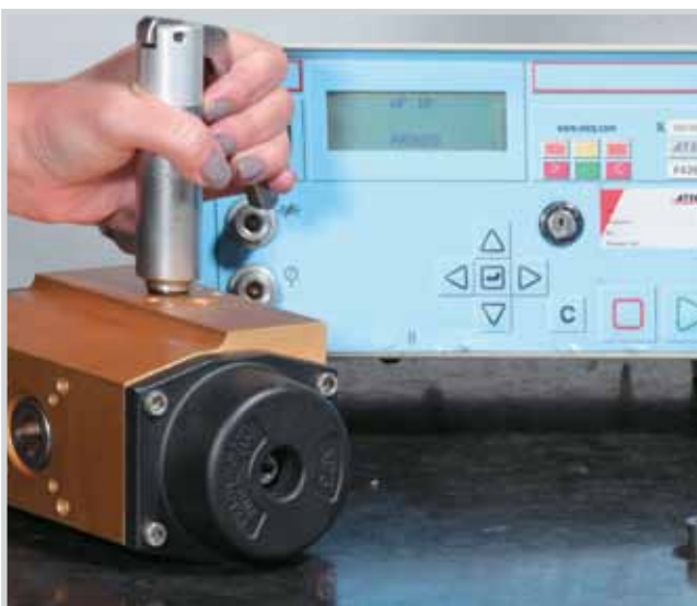
Leack test machine. For pneumatic rotary actuators.
