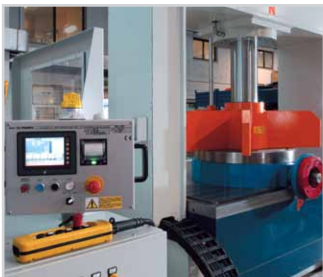
Vertical idraulic test machine. For butterfly and ball valves.
