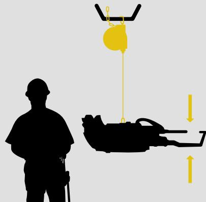
Kromer ATEX Balancers keep loads suspended reliably and safely at any height.
